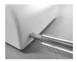
Repeat this process at the second lock. After that the front cover can be lifted from the mounting plate.
