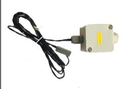
Metal probe with adhesive surface for measuring the temperature of photovoltaic modules. Comes with double-sided acrylic tape and cable length of 2m. The probe is supplied with a plastic box 50x52x35mm containing 4 to 20 mA transmitter. Necessary to set up KNX power supply and KNX analog input module acquisition.
