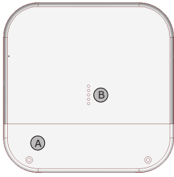
A. Cable compartment lid B. Operating indication LEDs
